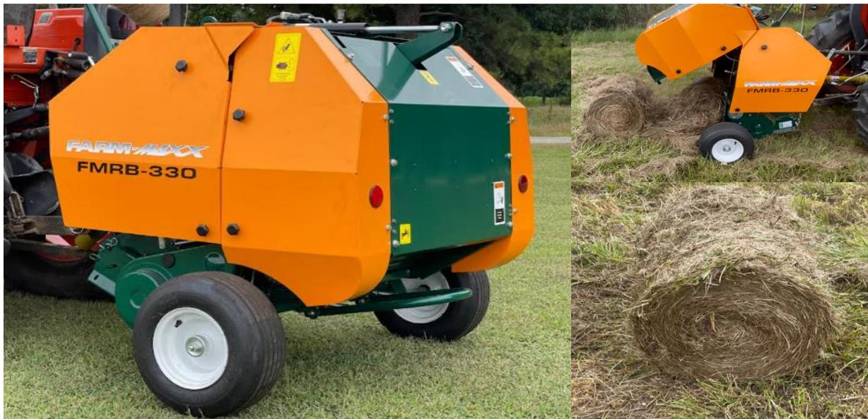
FMRB-330 Round Balers feature robust construction for years of trouble free baling. The superior design and simple plug & play hook-up means no messy hydraulic hoses. This makes these twine balers perfect for the small farmer in a hurry. Hay, straw, forage, even pine straw are no problem for this machine. Just connect your tractor to the three point hitch, plug in the wiring harness and off you go!
